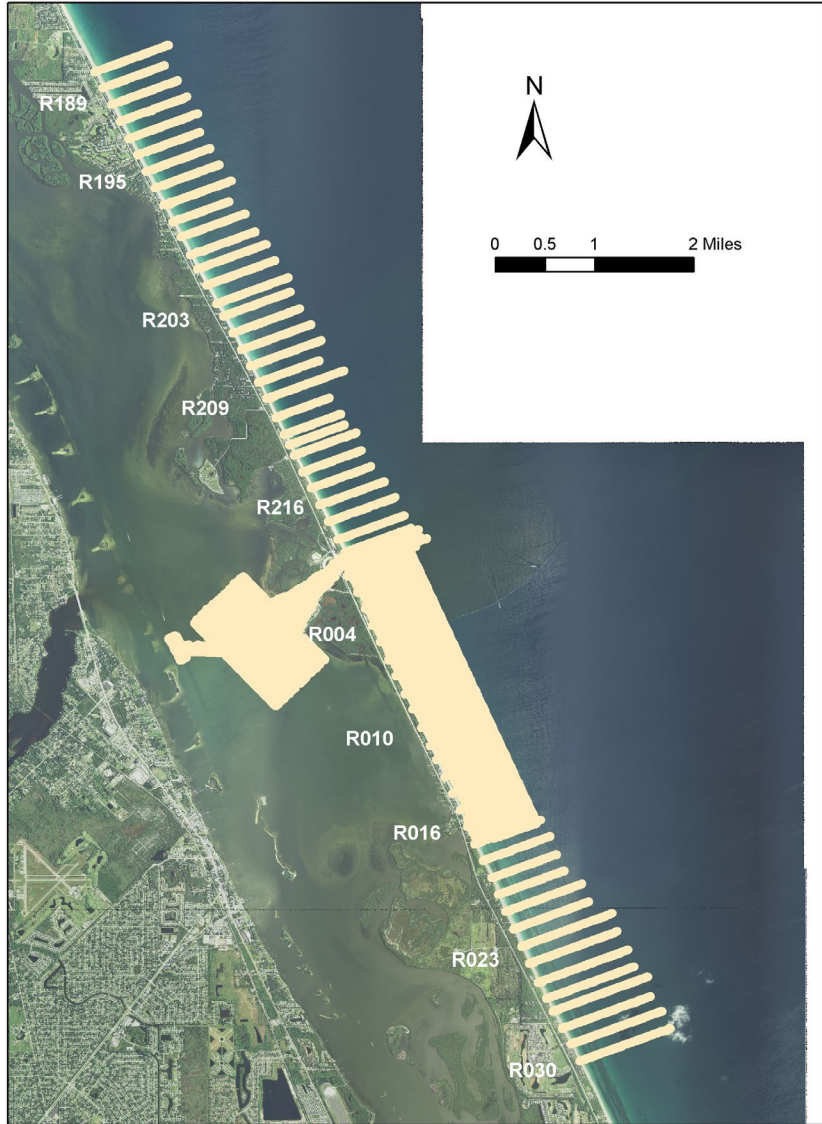
Figure 1. Typical Extent of hydrographic survey (2019 winter).
